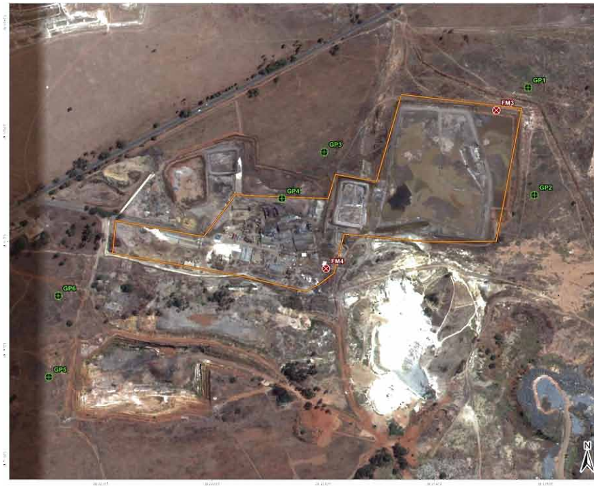
MONITORING BOREHOLE LOCALITY MAP
