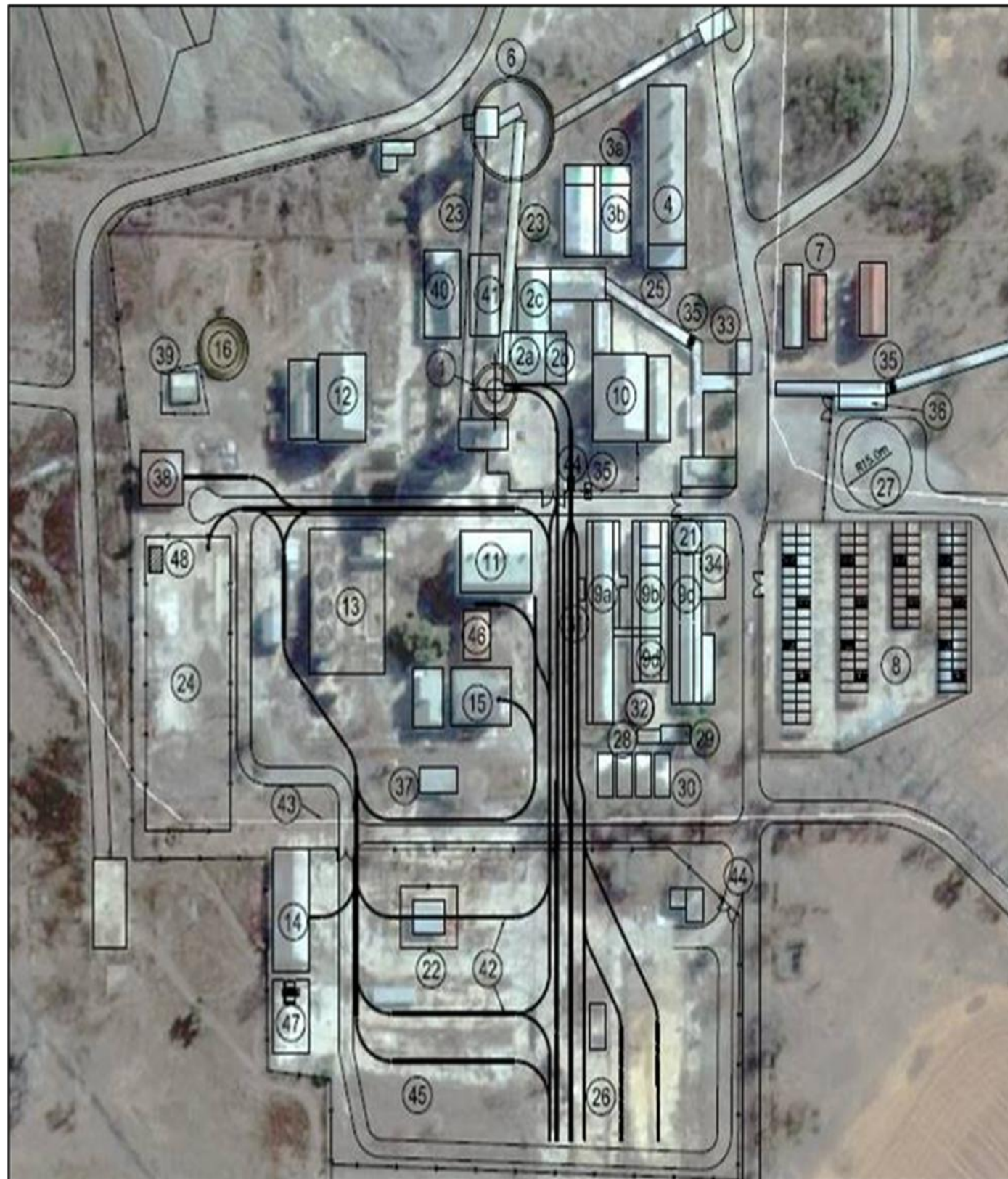
Figure 2-5: Target No 3 Shaft surface Infrastructure Layout
