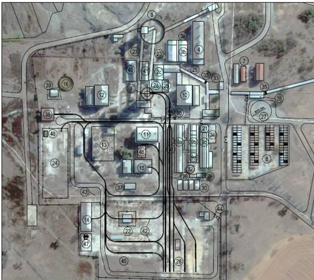
Figure 3: Target No 3 shaft surface infrastructure layout
