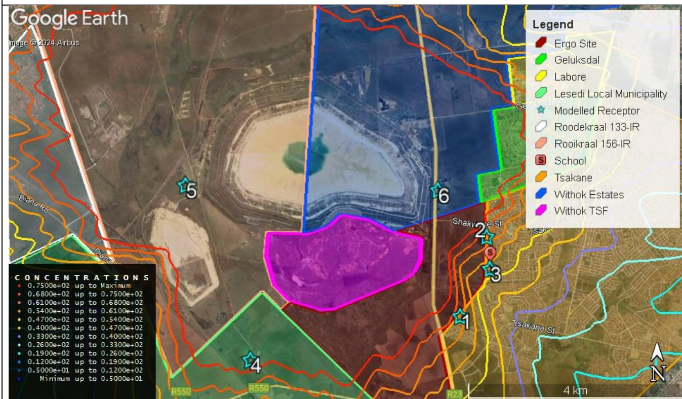
Figure 8-25: Modelled prediction of highest 24-hour average PM 10 concentrations resulting from emissions from the worst-case Brakpan TSF scenario.
