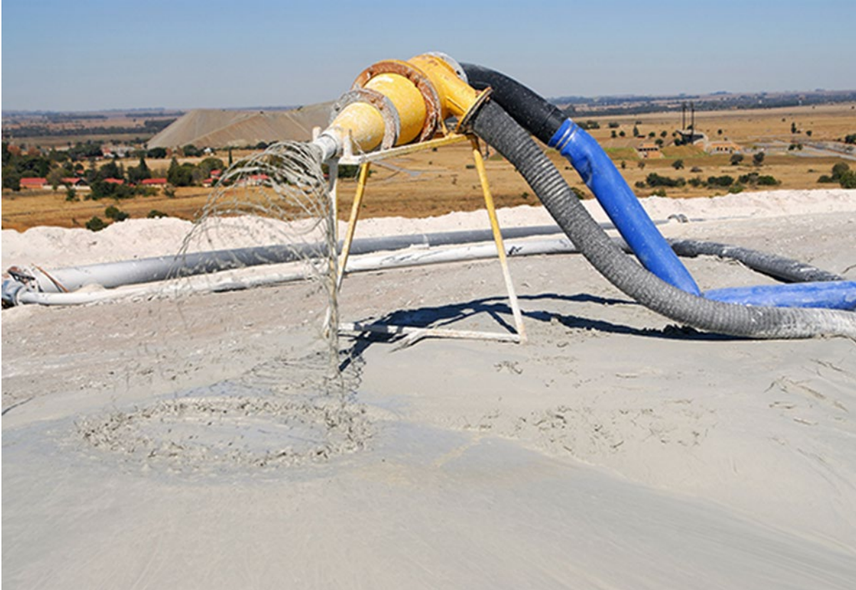
Figure 7-2: Illustration of "overflow" and "underflow" (©Gold Fields Limited, 2024).
